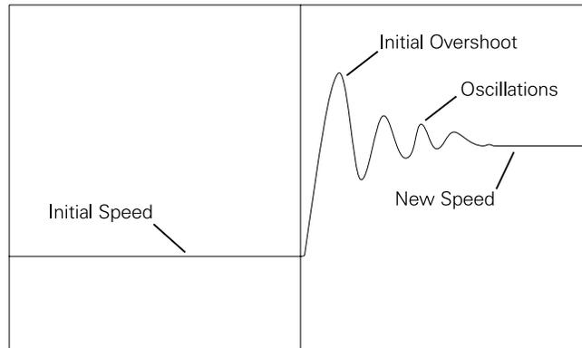
When the inertia of a system is properly matched the system will settle into a new speed quickly. This provides a stable system with quick response.
