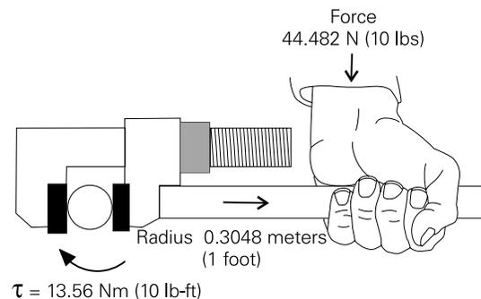
An increase in force or radius would result in a corresponding increase in torque. Increasing the radius to 0.6096 meters (2 feet), for example, results in 27.12 Nm (20 lb-ft) of torque.
