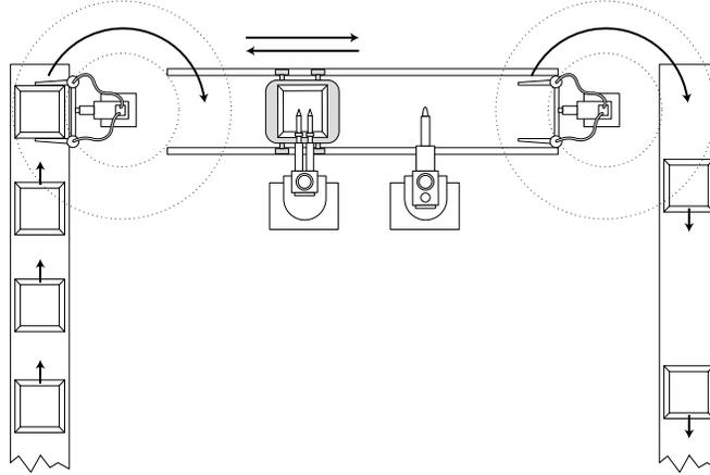
A rotational axis application has an endless traversing range. A rotary table, for example, travels along the shortest path from one point to the next. A rotary table may also have selectable or predefined directions of rotation to move from one point to the next.
