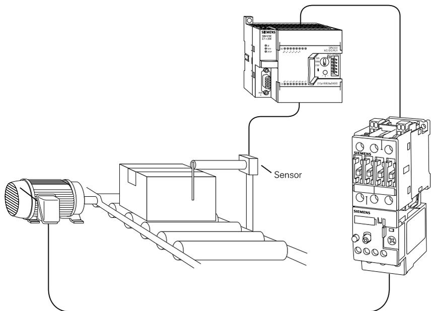
Another application might involve the use of an AC drive, such as a Siemens MICROMASTER, MIDIMASTER, or MASTERDRIVE. In this example a PLC is used to control a trimming cycle for a continuous roll. A sensor, connected to a PLC input, is used to detect a reference mark on the roll. An AC drive, controlled by the PLC, is used to control the acceleration, deceleration, and speed of an AC motor.
