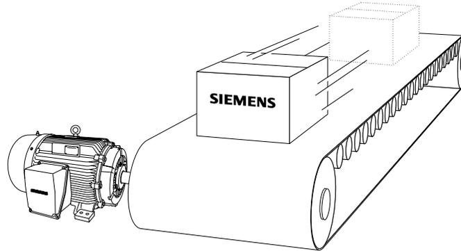
Work is defined by the product of the net force (F) applied and the distance (d) moved. If twice the force is applied, twice the work is done. If an object moves twice the distance, twice the work is done.
